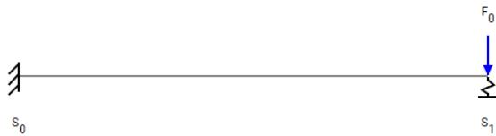
Test rotational spring, find moment  $M$  at support  $S_0$  with  $M = \frac{3Fl^2k_r}{16(3EI+k_rl)}$
